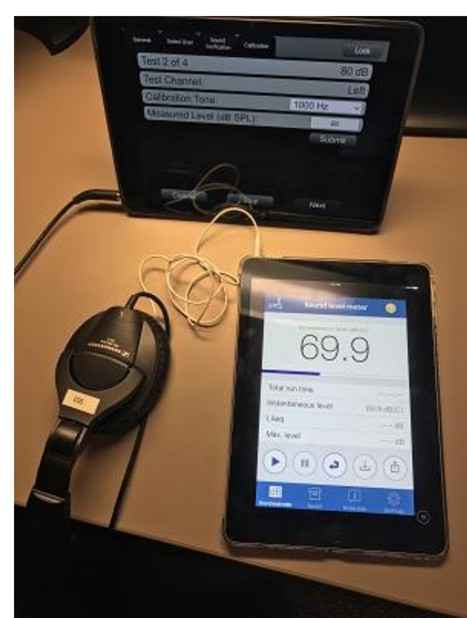
Figure 2. Routine calibration was conducted using the iBoundary microphone shown in Figure 2, and the NIOSH Sound Level Meter application, running on a second iPad. Initial calibration of the system and the NIOSH SLM application was conducted using the B&K system.
